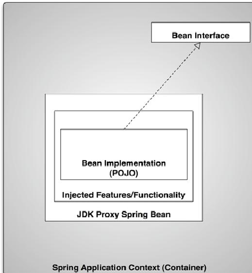
Spring-managed components are typically "Plain Old Java Objects" or POJOs. These application classes generally do not need to implement special interfaces or extend base classes, or be aware of the container they are running in. This facilitates writing portable and reusable code. However, developers may still hook into component and container lifecycles where needed.
